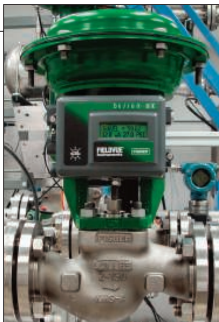
FIGURE 5. This compact chemical-service control valve is equipped with an integrated digital valve controller that features non-contact, linkage-less technology
